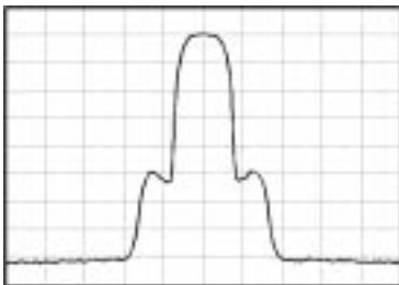
PHS Spectrum F_c = 1907 \text{ MHz} Span = 2 MHz Scale = 10 dB/div Level = +4 dBm
